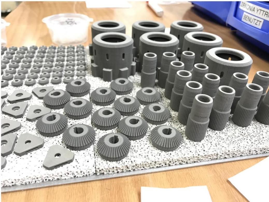
*Tritone highly robust green parts with low sintering shrinkage*
