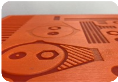
A printed mold layer prior to filling with paste
