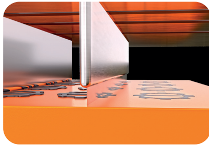
Paste being applied into mold cavities, b: the build layer after cavities are filled and dried.
