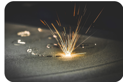
An observer of the LPBF process can see the sparks and smoke plume as the laser works its way across the powder bed.
