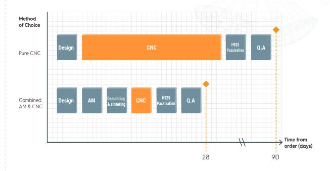
After comparing both options, CNC, and a combined AM & CNC approach, AMT Metal concluded that the combined AM & CNC method offered a quicker and more cost-effective solution.
