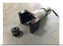
8. Unscrew the three marked bolts using the 2.5mm Allen key to remove the motor from its bracket.
