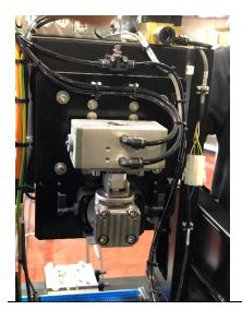
2. Unscrew the two marked bolts using the 4mm Allen key.
