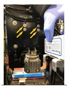
5. Once the motor is free of its bracket, remove the belt from the sprocket and then disconnect the Molex connector.
