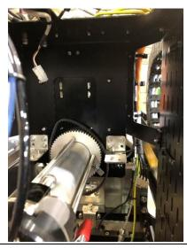
7. Disconnect the paste level sensor and the air supply hose.
