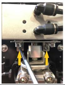
3. Put the valve aside to reveal the four bolts behind it.
