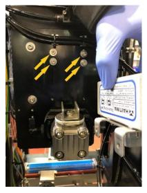
5. Once the motor is free of its bracket, remove the belt from the sprocket, and then disconnect the motor Molex connector.
