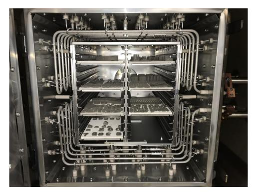
Tritone MoldJet parts ready for processing in an Elnik Furnace at DSH Technologies
