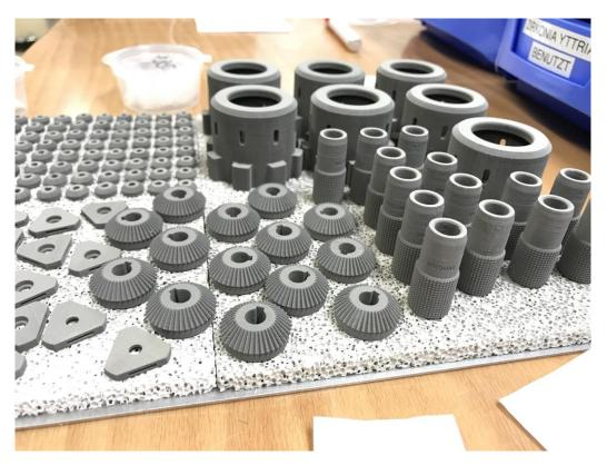
Tritone highly robust green parts with low sintering shrinkage
